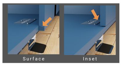
At least 2" (51mm) of flat toe kick space in the overhang for cabinets with surface mount cabinet door. For inset doors, add the door thickness to the 2" (51mm) requirement. Example: If the inset door is .5" (13mm) thick, the minimum toe kick depth required would be 2.5" (64mm). This is necessary to make sure the cabinet door and pedal mounting plate do not bind.
