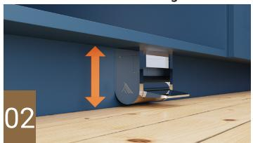
At least 3.25" (89mm)of toe kick height is required. Measure from the floor up the vertical toe kick face to where it intersects with the cabinet base overhang.
